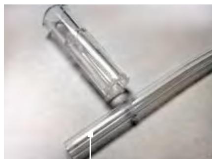
Tubing delaminates from luer.
