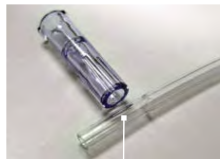
Tubing delaminates from luer.
